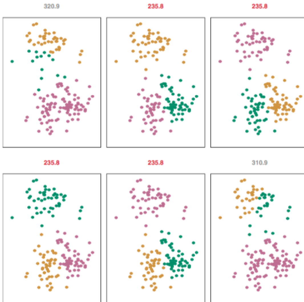
ISLR Figure 10.7: Different starting points can lead to different local minima
