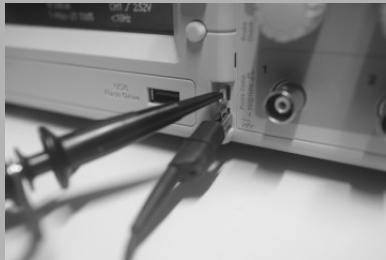
Figure 2: Connection of a probe for calibration. Figure 3: Adjustment of probe calibration.
