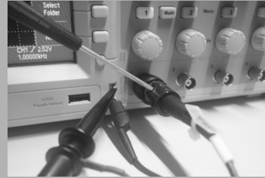
Figure 2: Connection of a probe for calibration. Figure 3: Adjustment of probe calibration.
