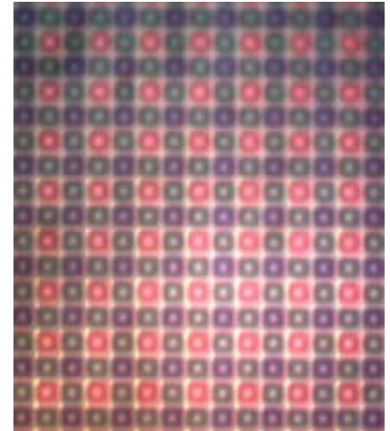
Below: The "retina" of the webcam and a close-up under a high magnification optical microscope.
