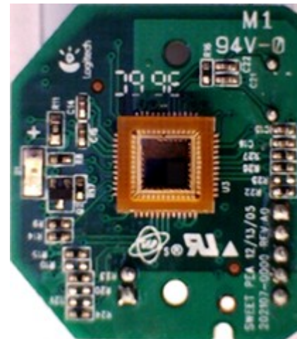
Below: The "retina" of the webcam and a close-up under a high magnification optical microscope.
