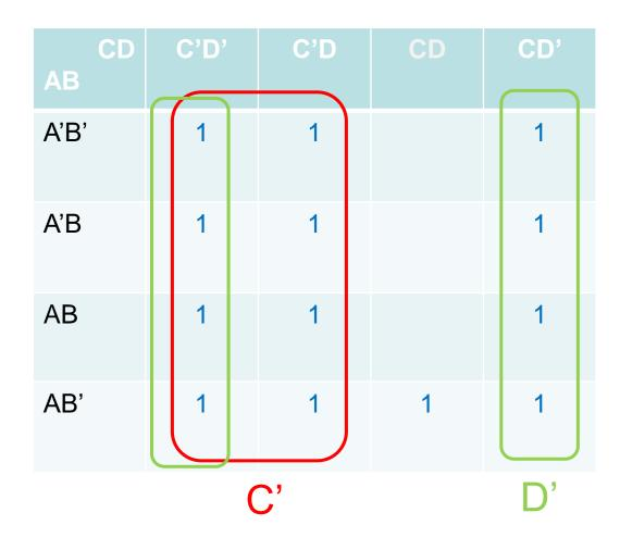
$y = C(\overline{A}\overline{B}\overline{D} + D) + A\overline{B}C + \overline{D}$
