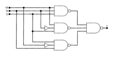
$X = \overline{M N Q} \cdot \overline{M N Q} \cdot \overline{M N Q}$   $X = M N Q + M \overline{N} Q + \overline{M} N Q$  X = MQ + NQ X = Q(M + N)  $M \longrightarrow Q$   $Q \longrightarrow X$
