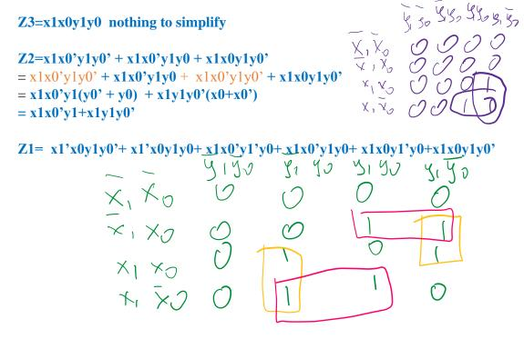
Z1 = x1x0'y0+x1y1'y0+x1'x0y1+x0y1y0'= x1y0 (x0'+y1')+x0y1 (x1'+y0')
