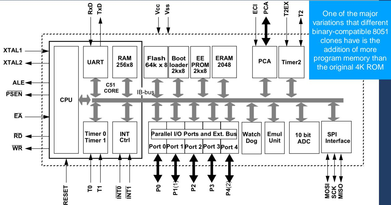
C8051F020 variant of 8051: 256 bytes of RAM C8051F020 variant of 8051: 64KB of Flash ProgMem
