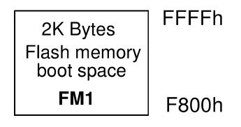
FM1 mapped between FFFFh and F800h when bit ENBOOT is set in AUXR1 register
