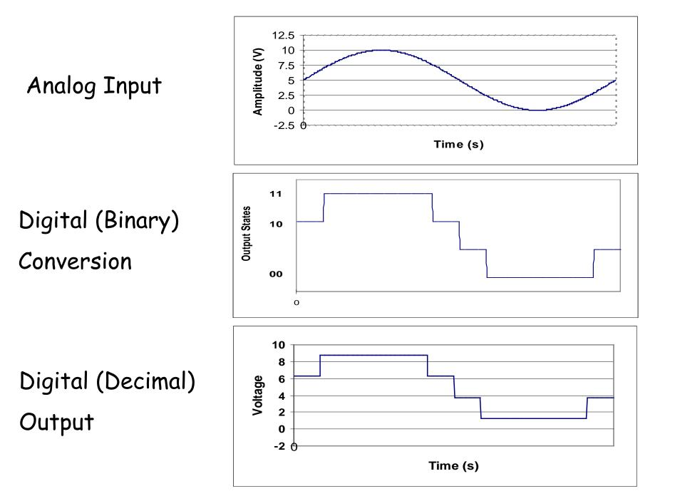
We now have a (pretty poor) representation of an analog input signal in digital (both binary and decimal) format.
