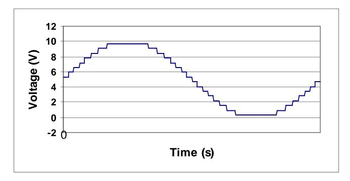
The number of different binary numbers that can represent the analog input =  $2^{no \ of \ bit}$  in each case.
