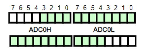
The mapping of the ADC0 analog inputs to the ADC0 data word registers is given by:
