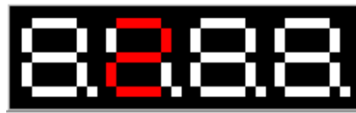
Fig 2.4 Digit 2 is shown at display 2
