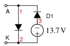
Zener diode subcircuit uses clamper (D1 and VZ) to model zener.
