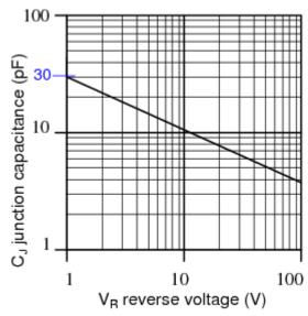
• If simulating high-speed transient response, as in switching regulator power supplies, TT and CJO parameters must be provided.
