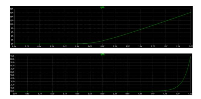
• Changing Da1N4004 model statement RS = 0  $\Omega$  to RS = 28.6 m $\Omega$  decreases the current at VD = 1.4 V to 12.2 A.
