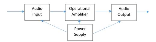
Keep the components in each section grouped together in the same area of the PCB to keep the conductive traces short. Long traces can pick up electromagnetic radiation from other sources, which can cause interference and noise.
