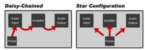
If sections are connected in a daisy-chain configuration, the current drawn from sections closer to the supply will create a voltage drop and result in lower voltages at sections further from the supply.
