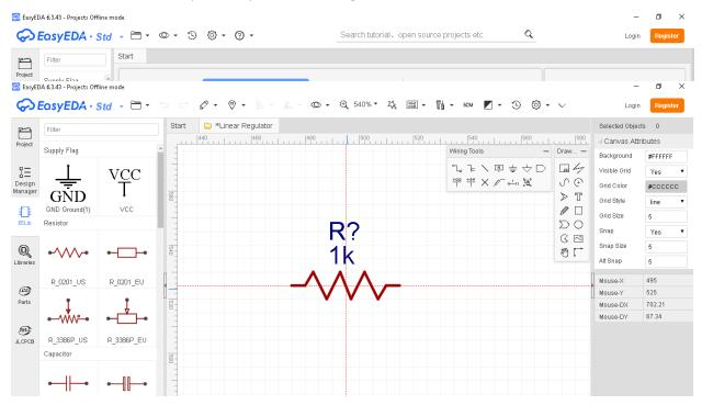
Once all of your symbols are placed on the schematic and you have assigned values to each symbol, it is time to start drawing the wires.
