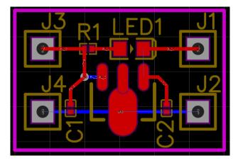
Notice that in the tracing given above the red traces are on the top layer and the blue traces are on the bottom layer. See also the via included to enable connection from the top layer to the bottom layer.
