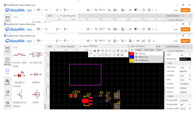
Notice the thin blue lines connecting the components. These are called ratsnest lines.
