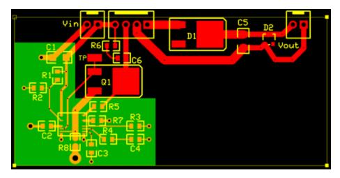
Ground layers are good for circuits that are prone to interference, because the large area of copper acts as a shield against electromagnetic fields. They also help dissipate the heat generated by the components.
