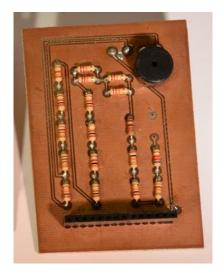
The copper thickness can vary and is specified by weight, in ounces per square foot. The vast majority of PCBs have 1 ounce of copper per square foot. But, some PCBs that handle very high power may use 2 or 3 ounce copper. Each ounce per square foot translates to about 35 micrometers or 1.4 thousandths of an inch of thickness of copper.
