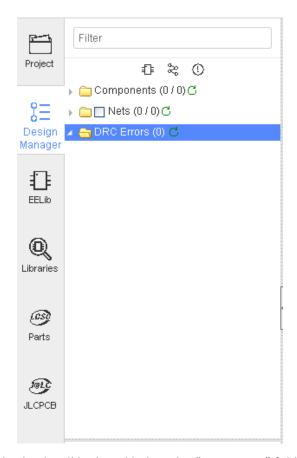
Items that fail the design rule check will be listed below the "DRC Errors" folder. If you click on one of the errors, the problem trace or component will be highlighted in the PCB view.
