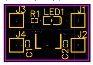
Add also PCB design texts to the PCB i.e. your name or team, date, version/revision, etc. (these texts could be attached on the top or bottom copper layer or on the silkscreen layer).
