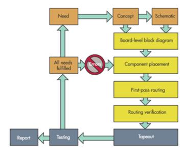
The concept includes the design's features, the functions the PCB must have and perform, interconnection with other circuits, placement, and the approximate final dimensions.
