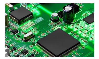
Solder is the metal that makes the electrical connections between the surface of the PCB and the electronic components. Being metal, solder also serves as a strong mechanical adhesive.
