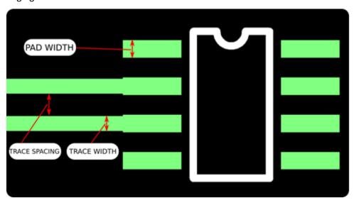
The proximity of traces to components and adjacent traces will also determine how wide your traces can be. If you are designing a small PCB with lots of traces and components, you might need to make the traces narrow for everything to fit.
