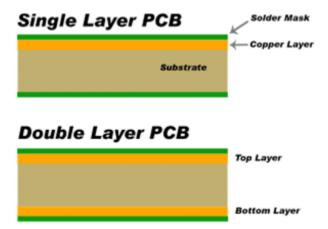
The traces on one layer can be connected to the other layer with a via. A via is a copper plated hole in the PCB that electrically connects the top layer to the bottom layer. You can also connect top and bottom traces at a component's through hole.
