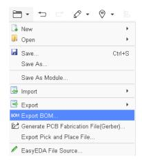
The BOM must be kept up-to-date with the schematic at all times. The BOM requires the quantity, reference designators, value (numeric value of ohms, farads, etc.), manufacturer part number, and PCB footprint for each component.
