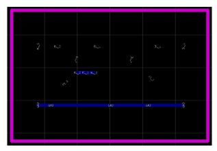
The top solder mask layer is shown in the figure below.
