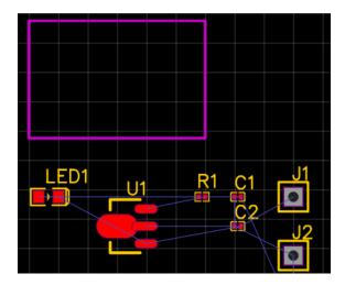
Now you can start arranging the components, keeping in mind the design tips mentioned in the previous section. You might want to do some research to find out if there are any special design requirements for your circuit. Some circuits perform better with certain components in specific locations. For example, in a linear voltage regulator circuit the decoupling capacitors need to be placed close to the chip to reduce noise.
