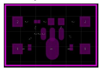
The bottom solder mask layer is as shown in the figure below.
