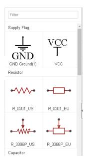
Each schematic symbol you use needs to have a PCB footprint associated with it. The PCB footprint will define the component's physical dimensions and placement of the copper pads or through holes. Now is a time to decide which components you will be using.
