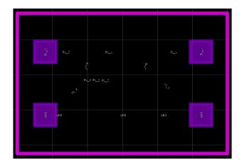
The figure shown below component outlines (silkscreen) layer of the PCB.
