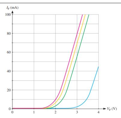
5. Develop a yellow LED traffic-light array using a minimum number of limiting resistors that operates from a 24 V supply and consists of 100 LEDs with  $I_F = 30$  mA and an equal number of LEDs in each parallel branch. Show the circuit and the resistor values. [12 marks]
