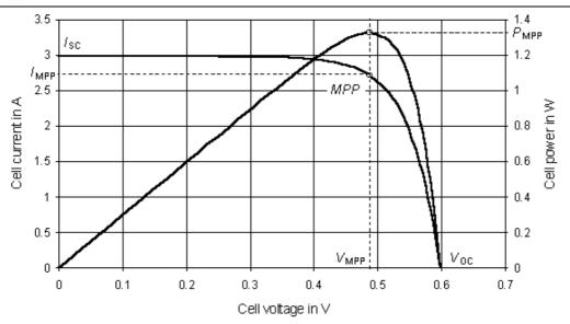
Use the MPP curve as given in the figure above to estimate and calculate the following design parameters specified for a solar power unit (note that the graph is based on the one solar cell characteristics instead of characteristics of a unit of cells):
