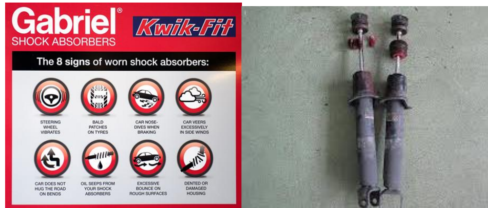
Figure 7: Worn out in the shock absorbers.
