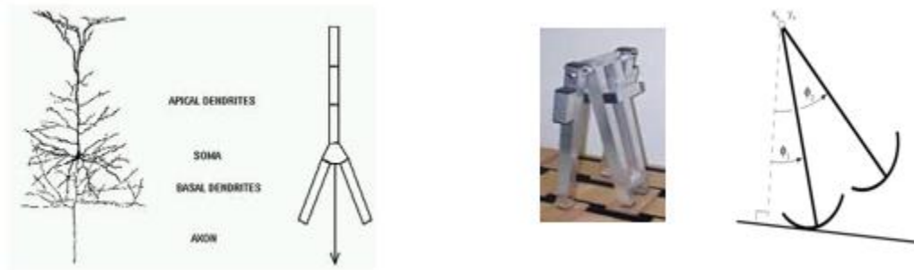
Figure 3: Lumped parameter model of a walking robot
