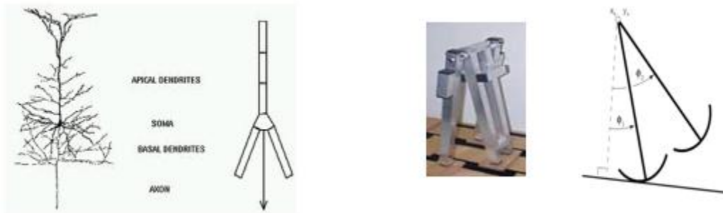
Figure 3: Lumped parameter model of a walking robot
