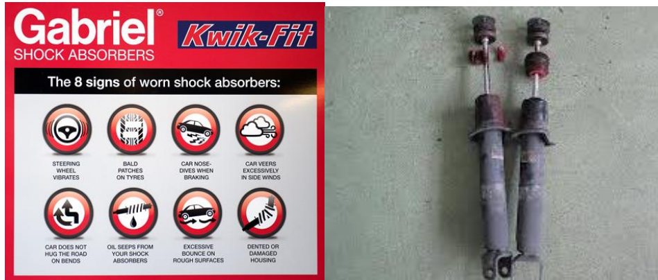
Figure 7: Worn out in the shock absorbers.
