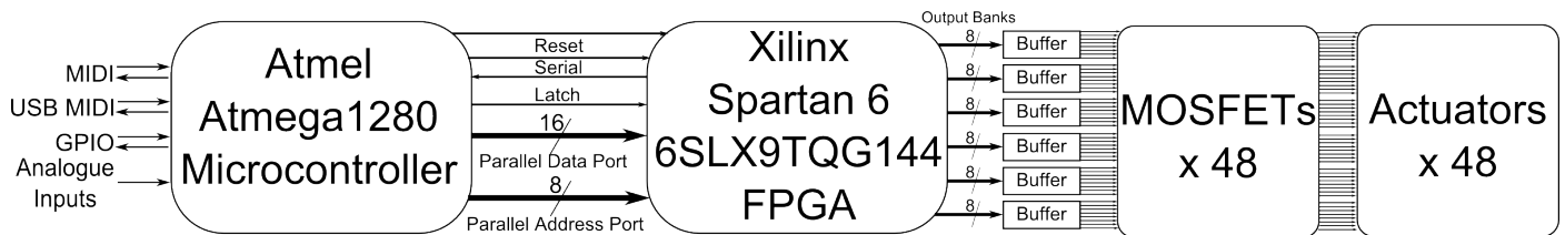
Fig. 3. Diagram of the robot controller circuit board's signal flow.
