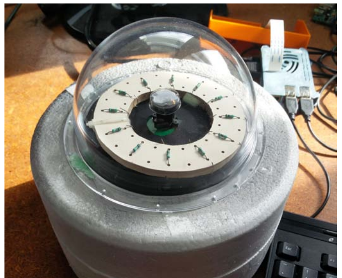
Fig. 4. First prototype skyPi showing resistive heater, and insulated enclosure.
