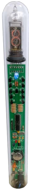
Fig. 4. The clock/frequency reference inside its glass-tube housing. The tube OD is 30mm and height is 300mm including the base. The single IN-14 display tube is at the top.
