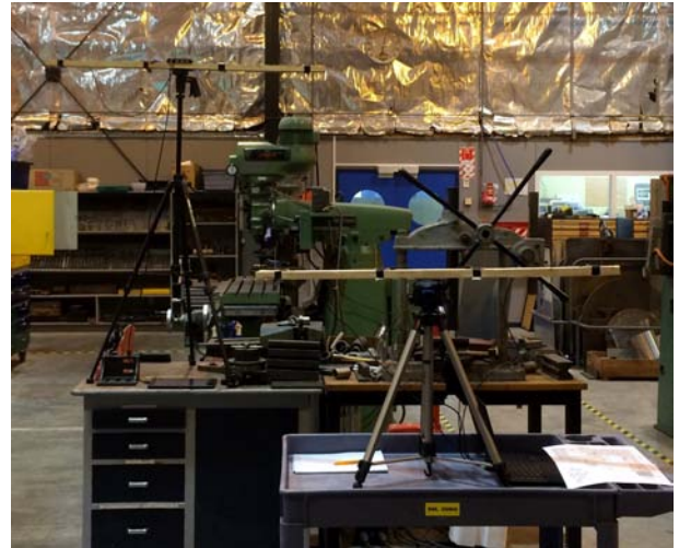
Fig. 3. Test mounts used, 'receivers' on table on left, 'transmitters' on mobile trolley on right
