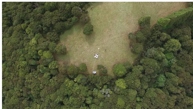
Fig. 7: Rural TART telescope site as seen from the drone during calibration flight. A battery powered noise source is attached to the drone and acts as a strong point source.
