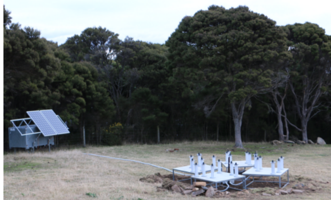
Fig. 1: Prototype of the TART deployed at the rural test site on Signal Hill, Dunedin. Telescope tiles with antennas on the right. The base station module as well as solar power system is placed within the metal box 15 meters away from the tiles.
