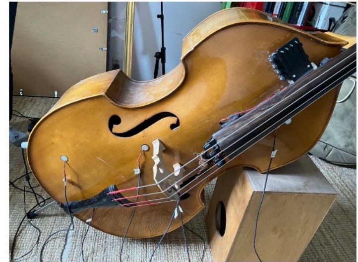
Figure 2. Piezo contact microphones attached at the front, tailpiece, bridge and inside the F-holes of the doublebass. The piezos at the back and on the scroll are not shown in the picture. The faders and knobs visible on the FAAB are used for individual string gain and effects blend (Melbye 2023: 81), respectively, for the FAAB's own signal processing. In the supplementary video and audio materials, no effects were used.
