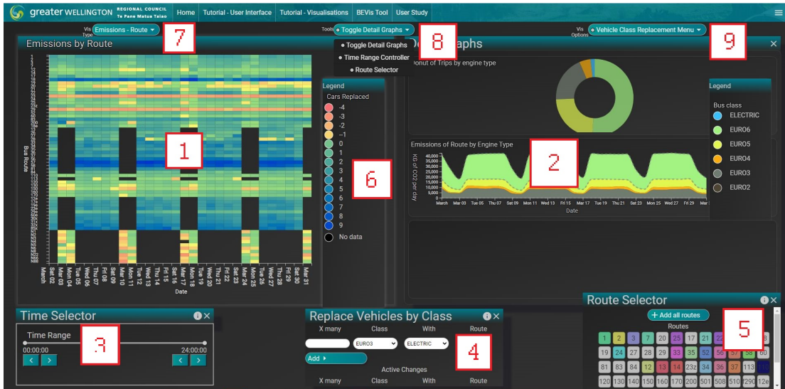
Figure 3.1: The final layout. 1. Main Visualisation window. 2. Detail Graphs window. 3. Time filter. 4. Replacement filter. 5. Route filter. 6. Legend window. 7. Visualisation selector. 8. Window controls. 9. Extra functions.
