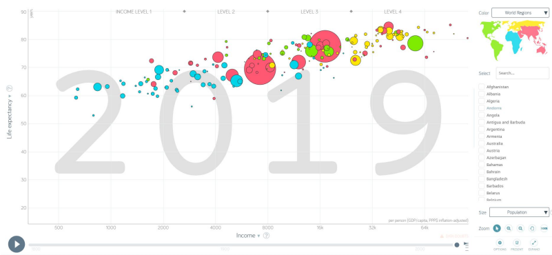
Figure 2.1: The GapMinder Bubble Chart showing life expectancy on the y vs income on the x. Each axis and the radius can be associated with different fields of interest in the dataset. The axis are controlled by the labels, the colour and radius can be set through the menu on the right.
