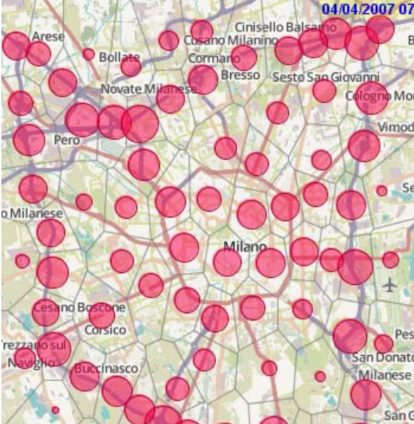
Figure 2.1: Sites on a map marked by circles which are sized according to the traffic throughput. [1]
