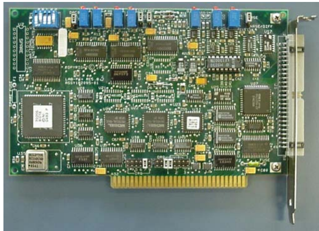
Figure 2.6: Lab-PC+ Data Acquisition Card
