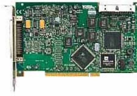
Figure 2.7: 6025E Data Acquisition Card
