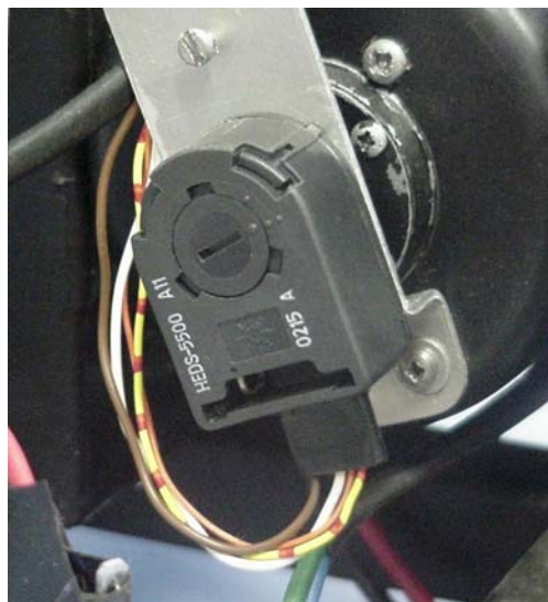
Figure 2.10: HEDS-5500 Optical Encoder Module
