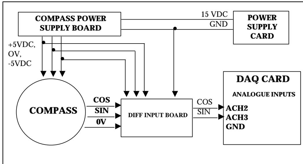
**Figure 4.2 COMPASS SENSOR HARDWARE CONFIGURATION.**
