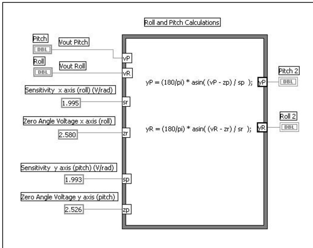
Figure 4.10 THE LABVIEW PROGRAM DEVELOPED FOR THE CXTA02 TILT SENSOR.
