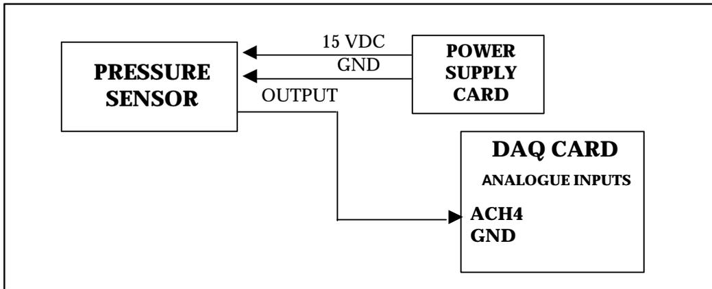
Figure 4.6 PRESSURE SENSOR HARDWARE CONFIGURATION.
