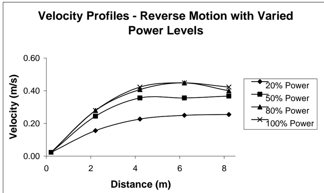
Figure 6.3 VELOCITY PROFILE OF THE ROV IN REVERSE MOTION.
