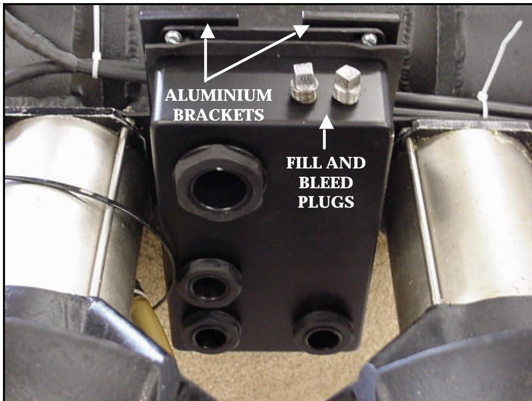
Figure 5.11 THE MOUNTING PLATES FOR THE JUNCTION BOX.
