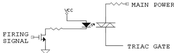
Figure 2.16 TRIAC FIRING CIRCUIT ONE.
