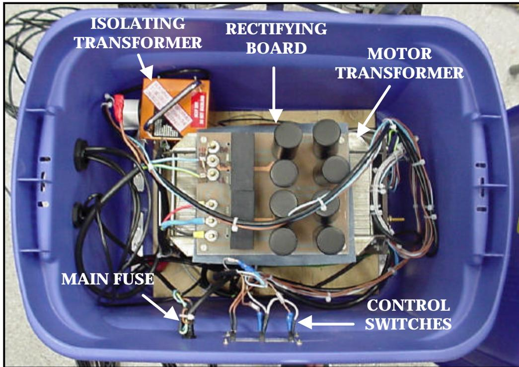
Figure 5.14 THE INTERNALS OF THE POWER BOX.
