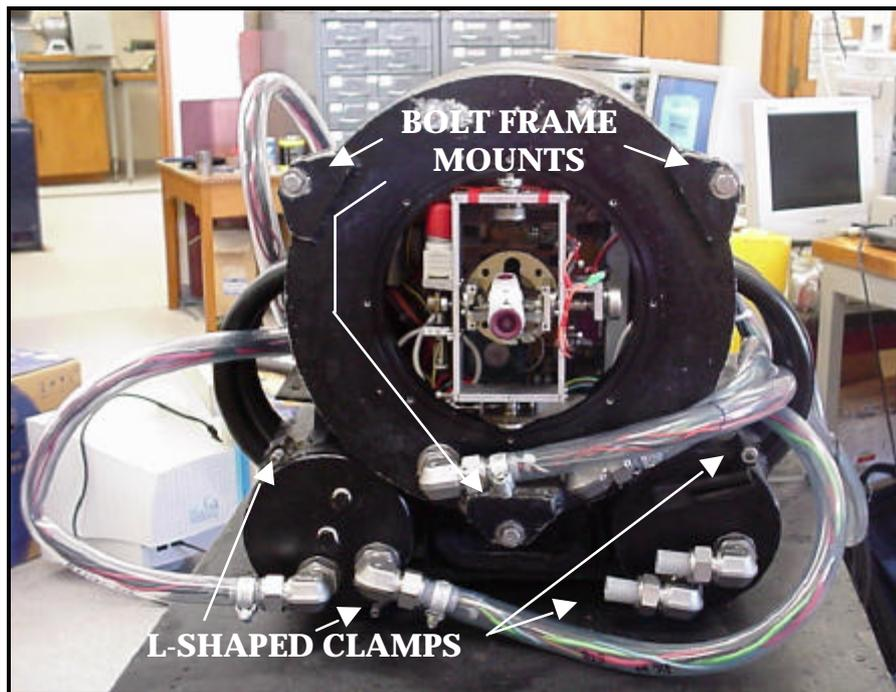
**Figure 5.17 THE PARTIALLY RECONSTRUCTED ROV.**
