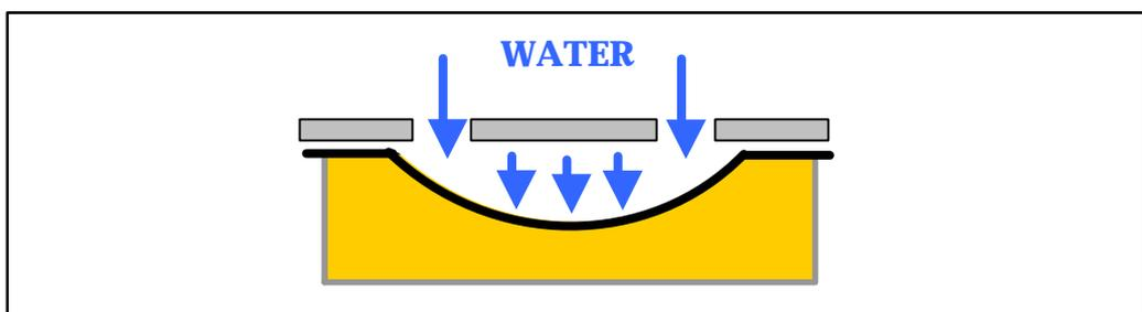
Figure 5.9 WATER COMPRESSING THE DIAPHRAGM.
