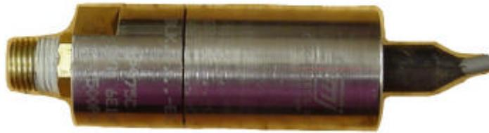
**Figure 3.16 THE BELL & HOWELL HIGH OUTPUT PRESSURE TRANSDUCER.**
