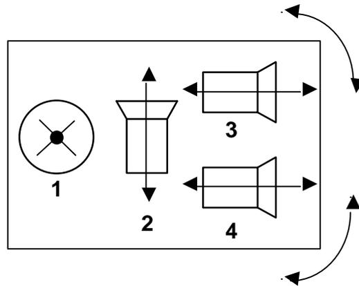
Figure 2.2 TOP VIEW OF THE THRUSTER LAYOUT AND DIRECTION OF MOTION.
