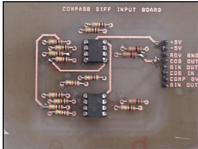
Figure 3.14 THE COMPASS DIFFERENTIAL INPUT BOARD.
