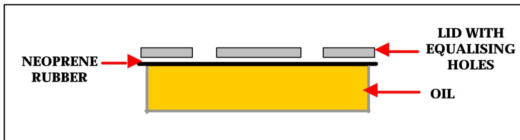
Figure 5.8 A CUT-AWAY VIEW OF THE JUNCTION BOX.
