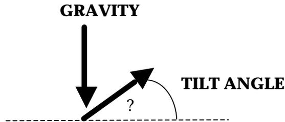
Figure 3.22 TILT ANGLE RELATIVE TO GRAVITY.
