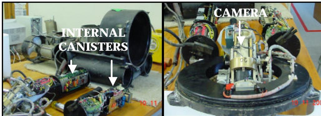
Figure 1.6 THE INTERNAL COMPONENTS OF THE DART ROV.
