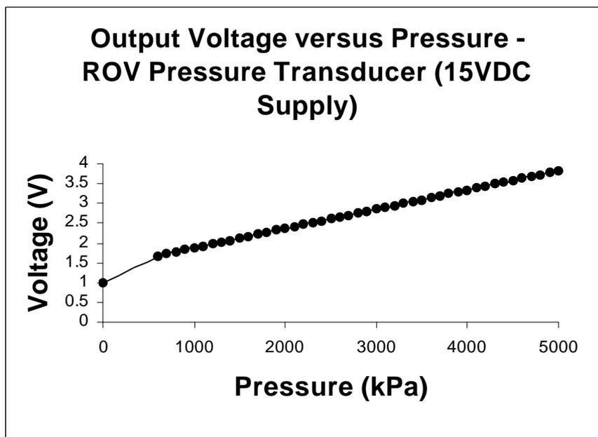
Figure 3.19 VARIATION OF THE BELL & HOWELL TRANSDUCER OUTPUT WITH PRESSURE.
