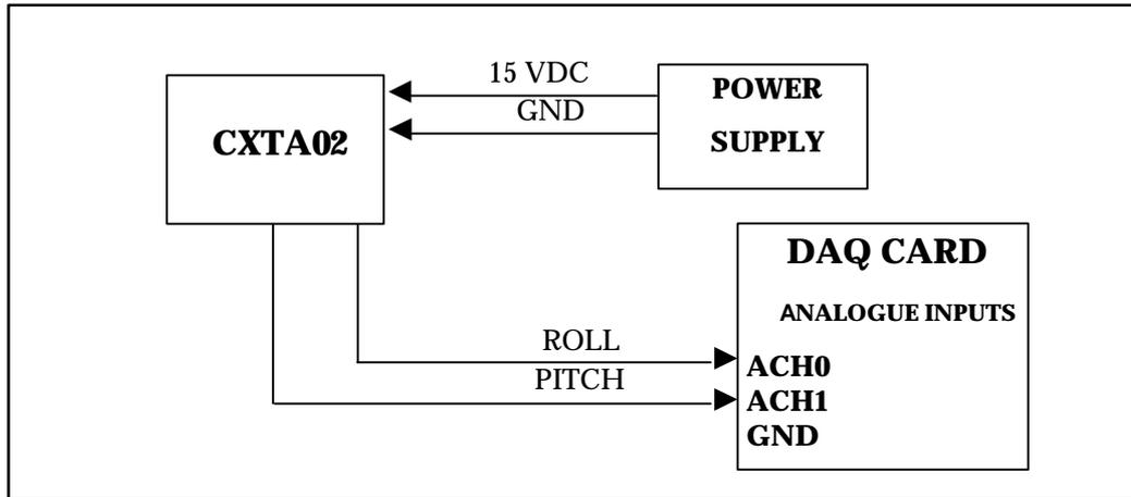
**Figure 4.9 TILT SENSOR HARDWARE CONFIGURATION.**
