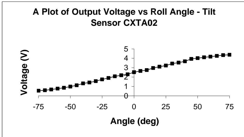
Figure 3.25 VOLTAGE RESPONSE OF THE CXTA02 SENSOR IN ROLL MOTION.
