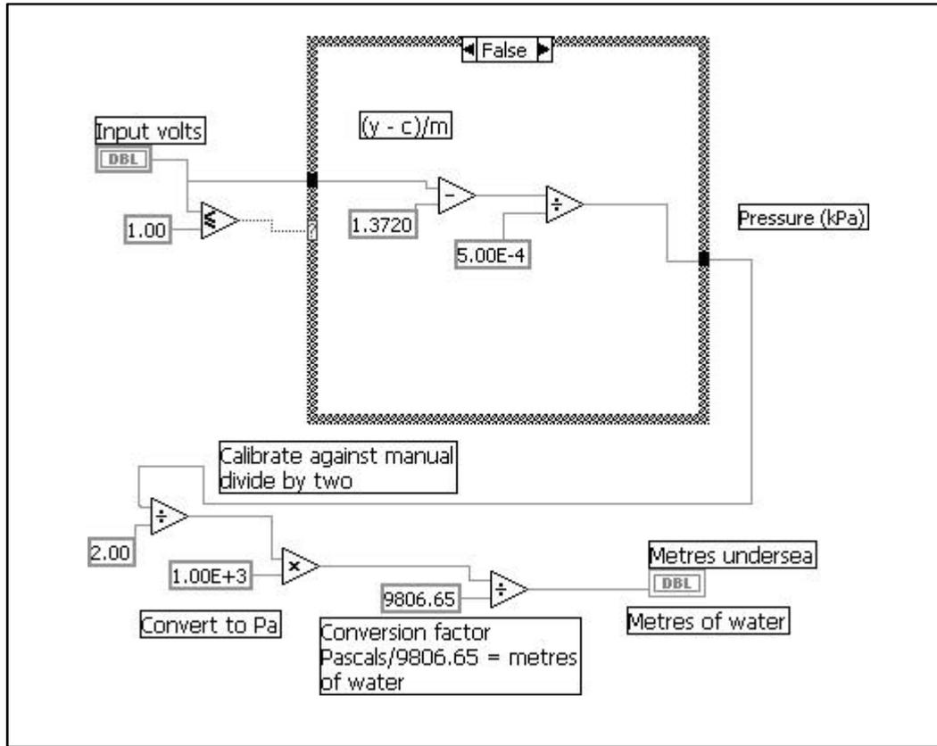
**Figure 4.7 THE LABVIEW PROGRAM DEVELOPED FOR THE PRESSURE TRANSDUCER.**
