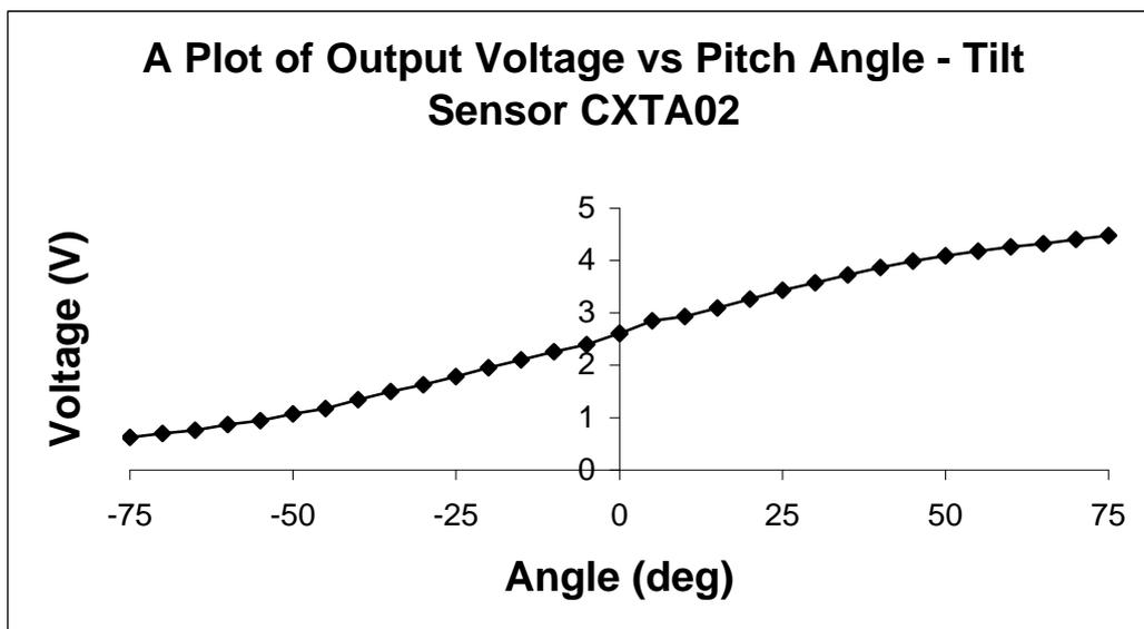
Figure 3.24 VOLTAGE RESPONSE OF THE CXTA02 SENSOR IN PITCH MOTION.
