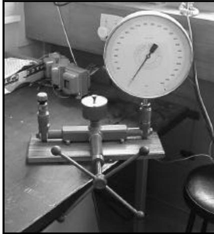
Figure 3.18 THE PRESSURE CALIBRATION APPARATUS.
