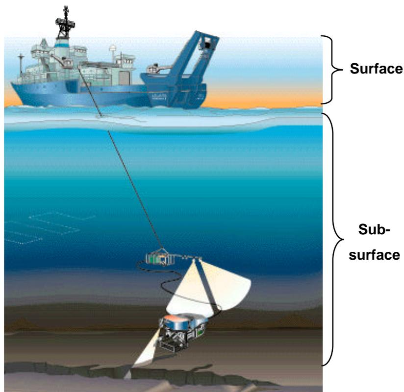
**Figure 1.4 THE SURFACE AND SUBSURFACE COMPONENTS OF AN ROV SYSTEM.**
