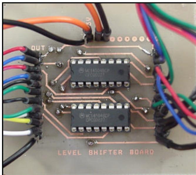
**Figure 3.8 THE LEVEL SHIFTER BOARD**
