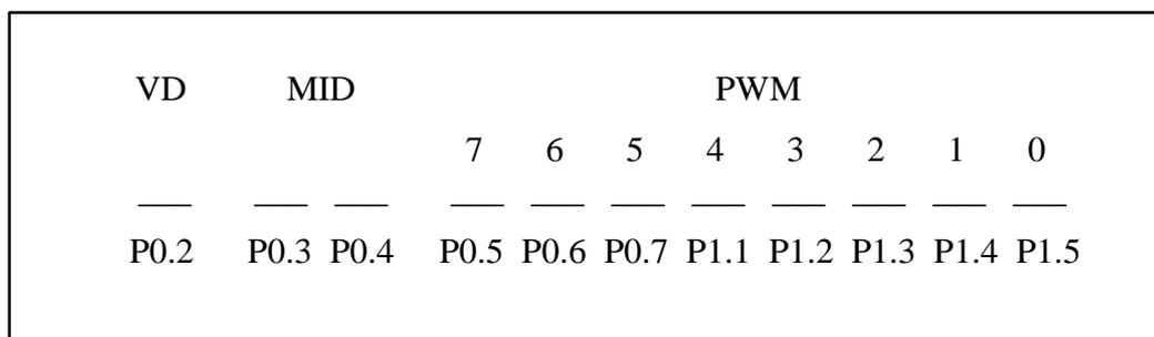
**Figure 4.15 ASSIGNMENT OF THE ELEVEN BIT WORD.**
