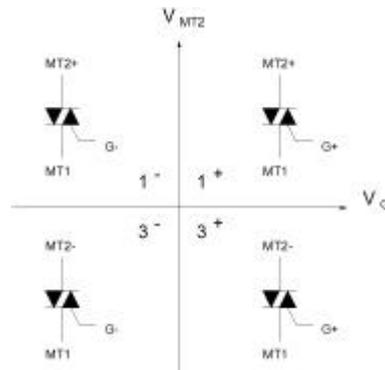
Figure 2.15 THE FOUR QUADRANTS OF TRIAC TRIGGERING.
