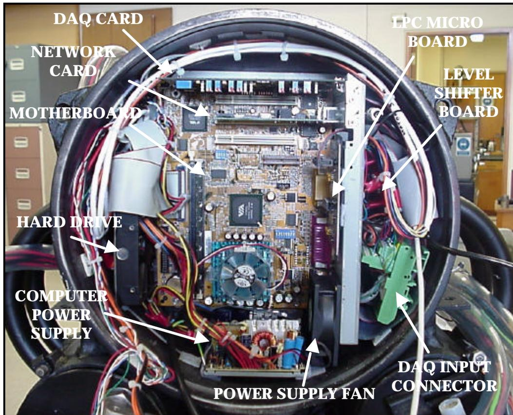
Figure 5.3 THE MAIN HULL OF THE ROV.
