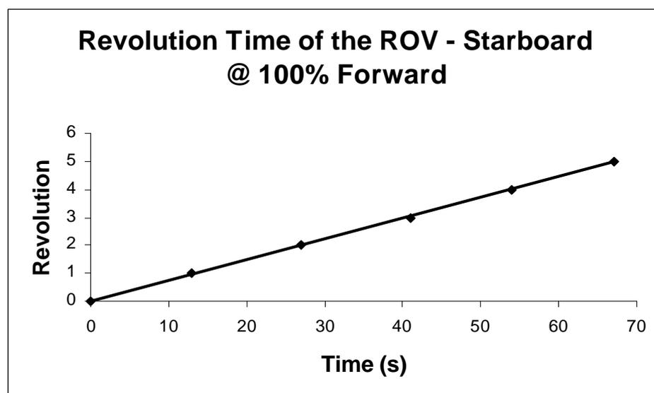
**Figure 6.5 ROV REVOLUTION TIME WITH THE STARBOARD MOTOR AT FULL POWER.**
