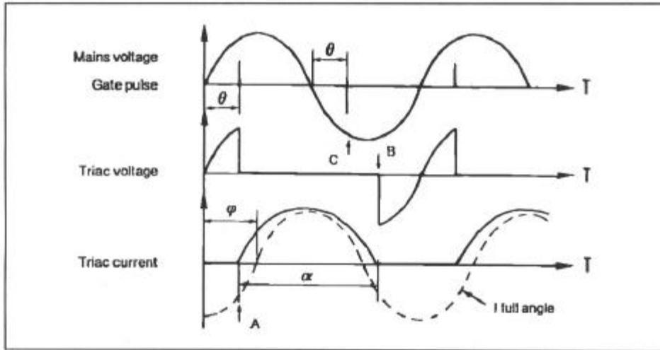
Figure 2.14 ASYMMETRICAL OPERATION OF A MAINS SYNCHRONISED TRIAC [7].
