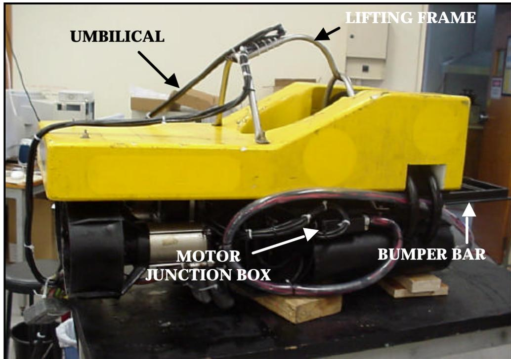
**Figure 5.18 THE RECONSTRUCTED ROV.**
