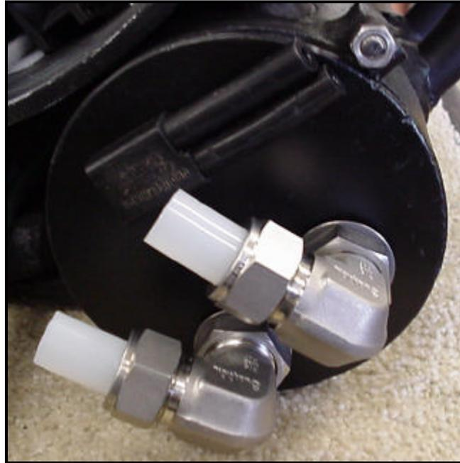
**Figure 5.13 THE NEW SWAGE-LOC FITTINGS AND WHITE NYLON-TUBING.**
