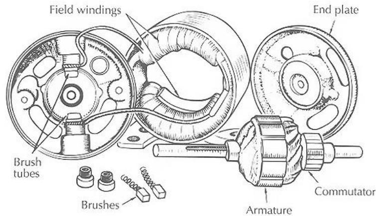
**Figure 2.3 THE COMPONENTS OF A UNIVERSAL MOTOR [3].**
