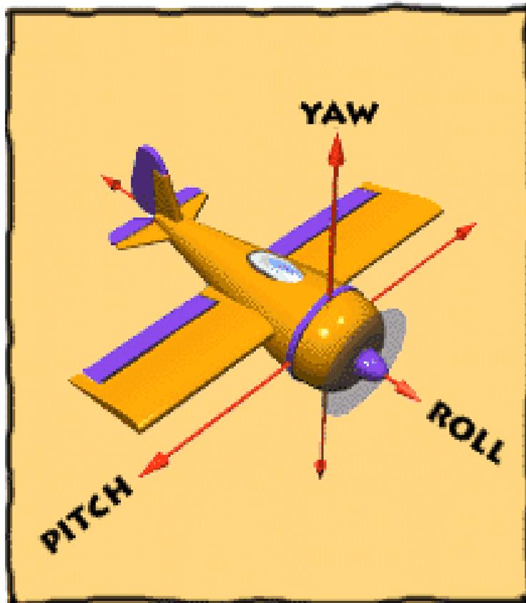
Figure 3.21 THE THREE AXES OF MOTION [15].
