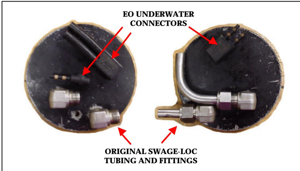
**Figure 5.12 THE ORIGINAL LAYOUT OF THE HULL CAPS.**
