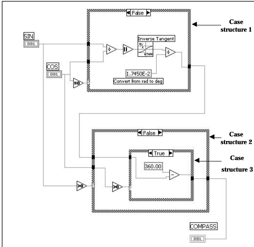
Figure 4.4 THE LABVIEW PROGRAM FOR THE WESMAR COMPASS.
