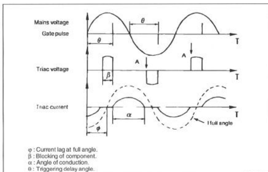
Figure 2.13 SYMMETRICAL OPERATION OF A MAINS SYNCHRONISED TRIAC [7].
