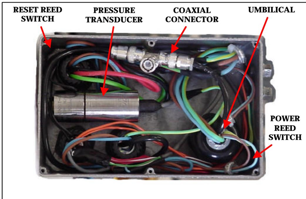
Figure 5.10 THE INSIDE OF THE JUNCTION BOX.
