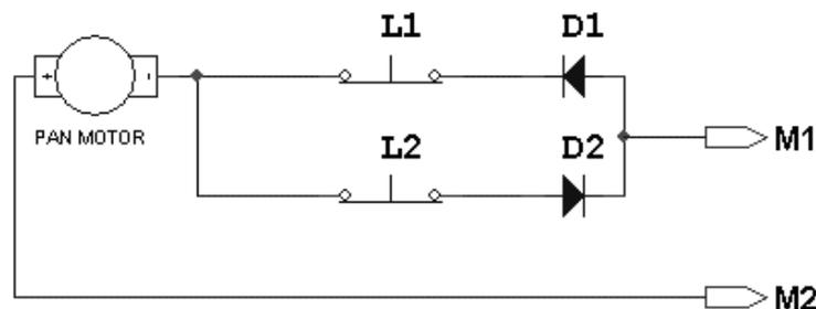
**Figure 3.28 THE PAN MOTOR CIRCUIT TO PROTECT THE DC MOTORS.**
