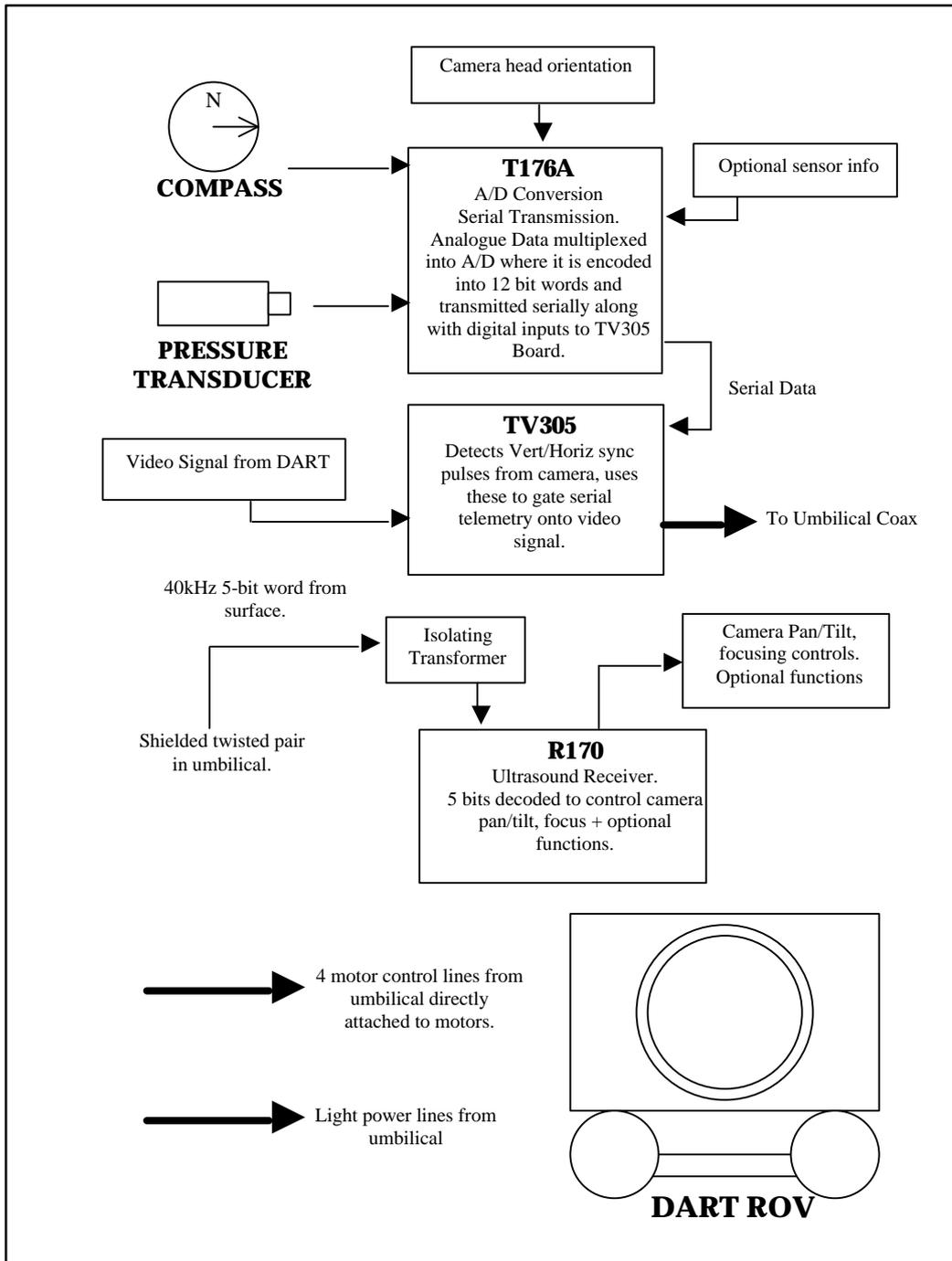
Figure 1.7 AN OVERVIEW OF THE ORIGINAL SUB-SURFACE COMPONENTS.
