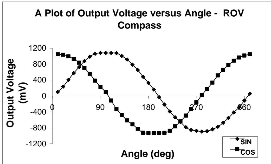
Figure 3.15 VARIATION OF THE SINE AND COSINE OUTPUTS OF THE DC700 WESMAR COMPASS WITH ANGLE.
