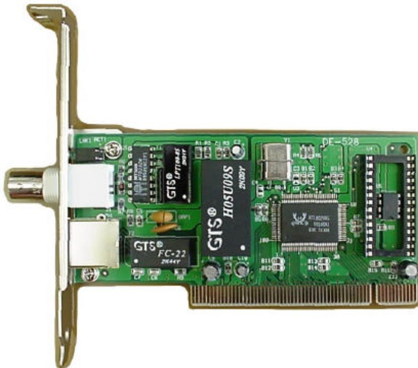
Figure 3.5 THE D-LINK DE-528 SERIES NETWORK CARD.
