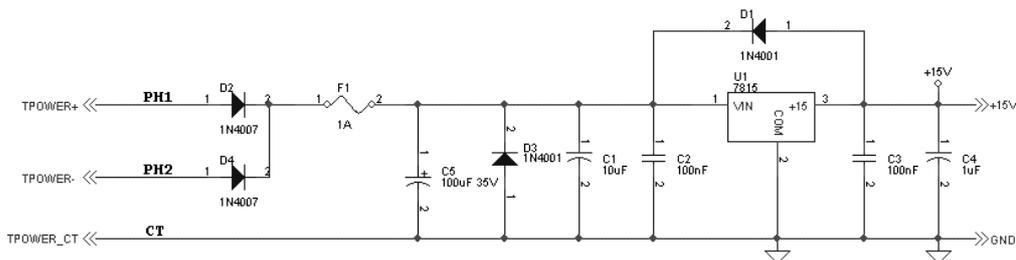
**Figure 2.27 THE POWER SUPPLY CARD SCHEMATIC.**
