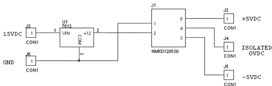
**Figure 3.11 THE COMPASS POWER SUPPLY BOARD CIRCUIT.**
