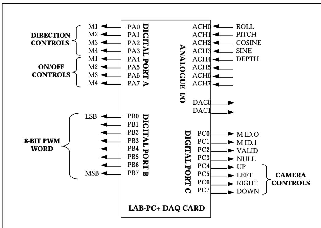
Figure 3.4 BLOCK DIAGRAM OF THE LAB-PC+ DAQ CARD.
