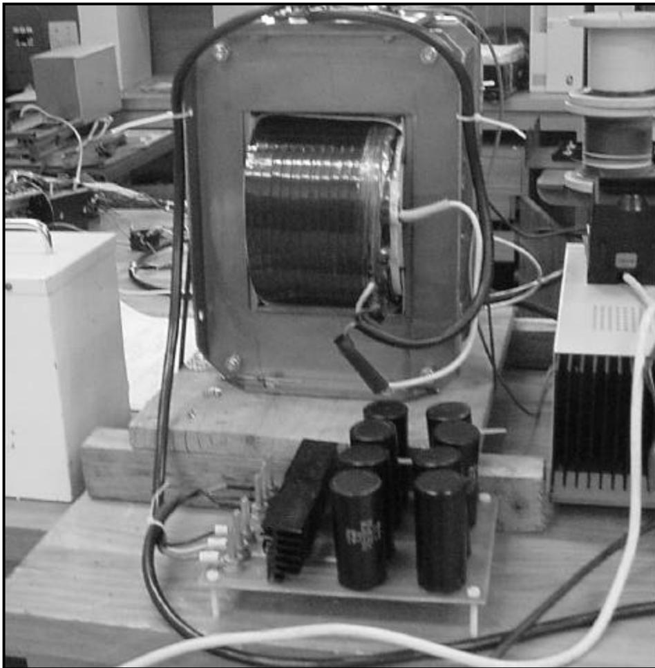
**Figure 2.25 THE MOTOR TRANSFORMER AND POWER RECTIFICATION BOARD.**
