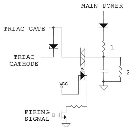
**Figure 2.17 TRIAC FIRING CIRCUIT TWO.**
