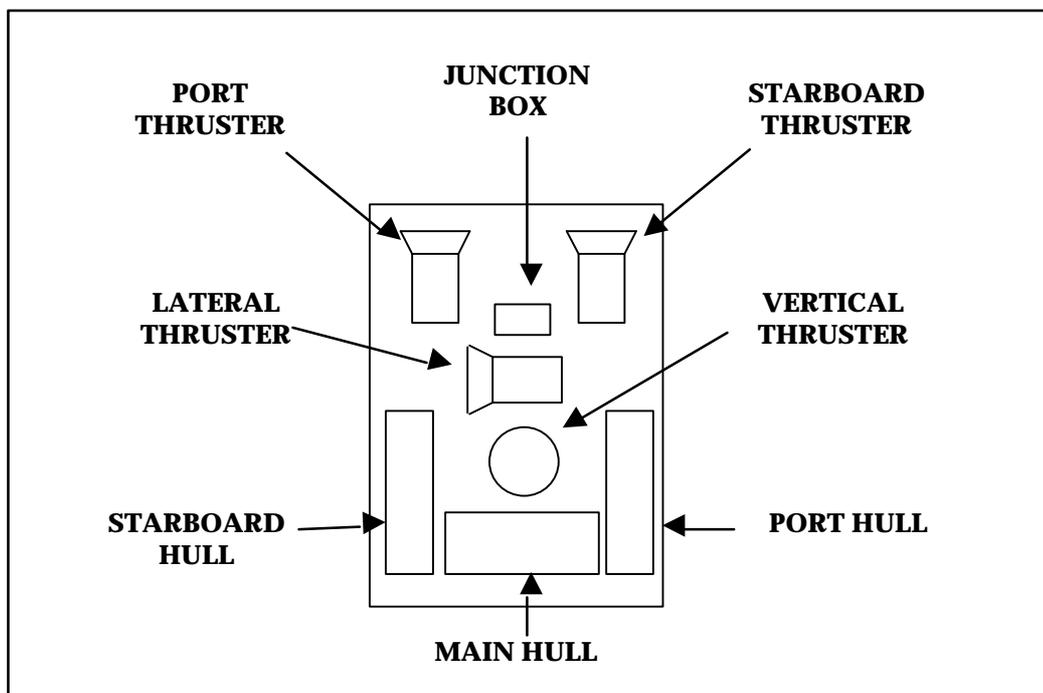
Figure 5.2 A TOP VIEW OF THE ROV.
