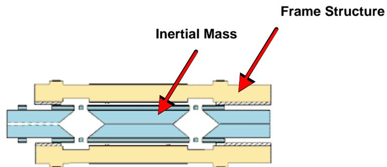
Figure 3.23 CROSS-SECTION OF A MICRO-MACHINED CAPACITIVE ACCELEROMETER [17].
