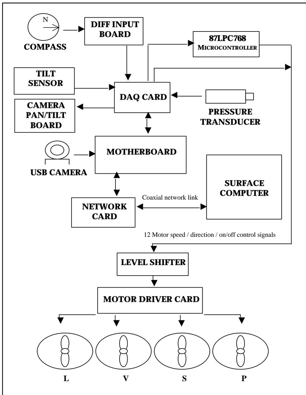
Figure 3.1 AN OVERVIEW OF THE NEW HARDWARE COMPONENTS.
