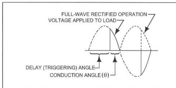
Figure 2.9 PHASE ANGLE CONTROL [5].
