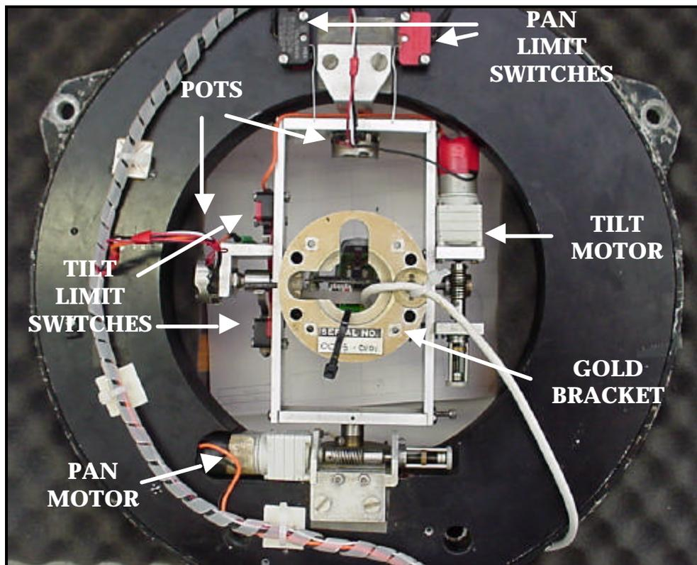
**Figure 3.29 A REAR VIEW OF THE CAMERA PAN AND TILT UNIT.**
