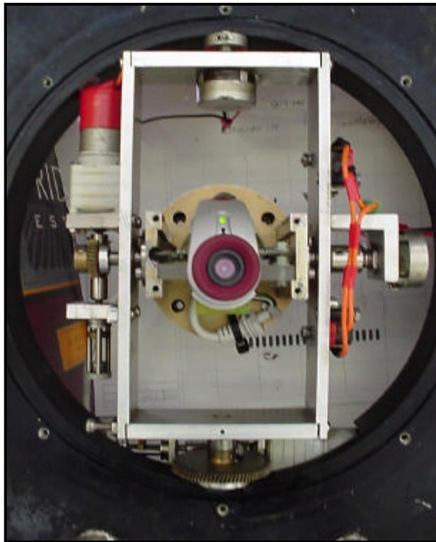
**Figure 3.31 THE PHILIPS USB CAMERA MOUNTED IN THE PAN AND TILT FRAME.**
