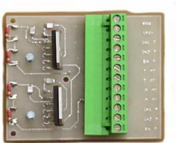
Figure 3.33 THE CAMERA PAN/TILT BOARD.
