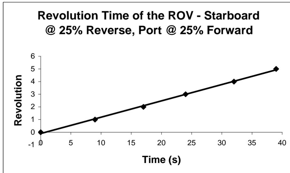
**Figure 6.4 ROV REVOLUTION TIME WHEN TWO MOTORS ARE POWERED IN OPPOSITE DIRECTIONS.**
