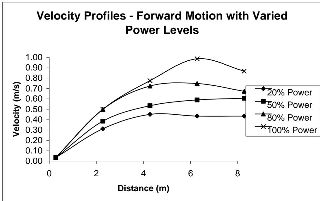
Figure 6.2 VELOCITY PROFILE OF THE ROV IN FORWARD MOTION.
