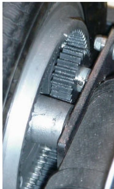
Figure 2-13: Standard drive configuration for an electric wheelchair
