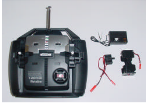
Figure 5-17: Two-channel radio control set
