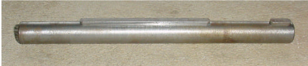
Figure 3-24: Track module drive shaft and corresponding keys
