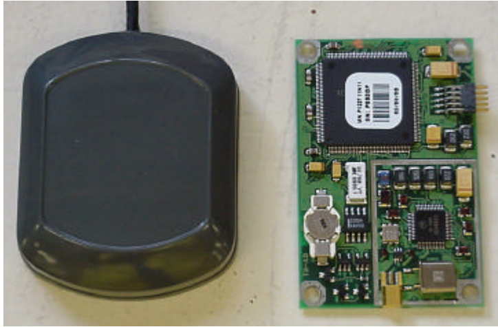
Figure 5-36: M12 GPS unit and antenna
