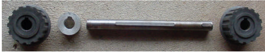
Figure 3-27: Drive shaft unit component layout
