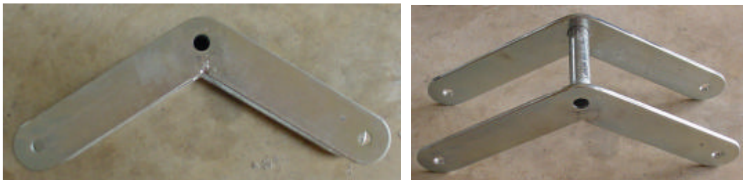
Figure 3-32: Completed track bogie unit frame
