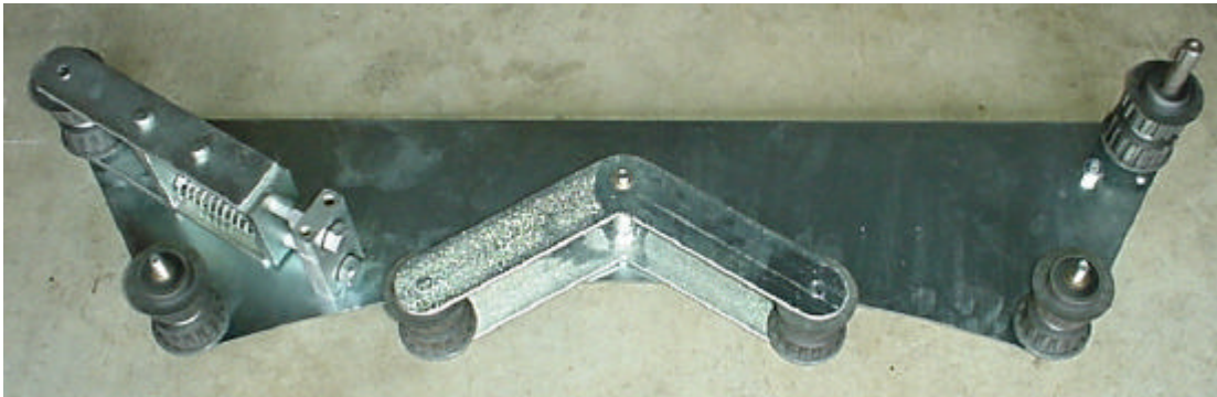
Figure 3-35: Exposed internal mechanisms of a track module
