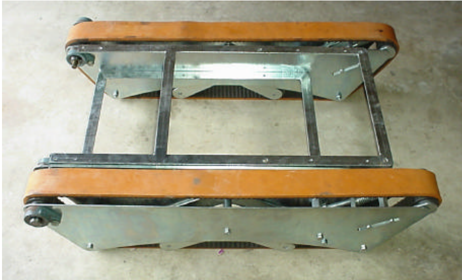
Figure 4-3: Assembled chassis trays and track modules
