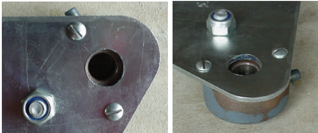
Figure 3-34: Inside of attached bearing flange
