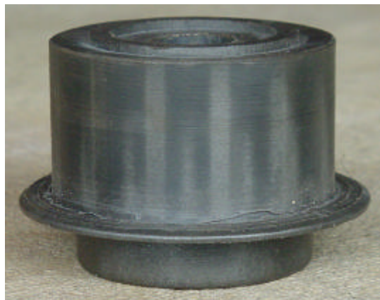
Figure 3-15: Guide pulley for static positions
