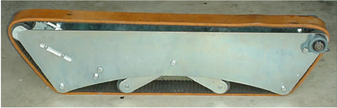
Figure 3-36: Assembled track module with tensioned belt
