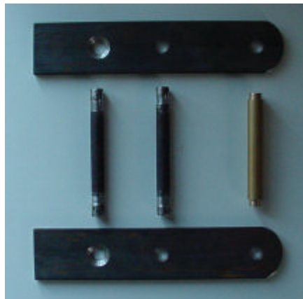
Figure 3-6: Component layout of the front sliding axle unit, prior to welding
