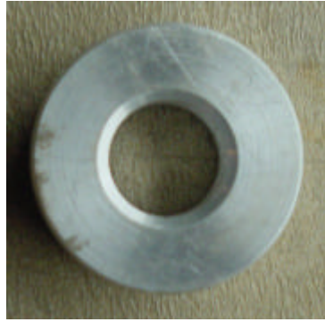
Figure 3-17: Aluminium spacers to separate all guide pulley units
