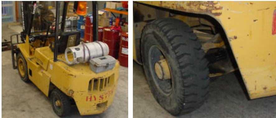
Figure 2-7: Forklift steering mechanism (rear wheel steering)
