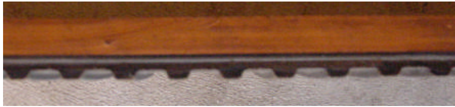
Figure 3-3: Side profile of the H-Type transmission belt (black), with an additional 10mm of high quality vulcanised rubber laminated to its outer face (orange)
