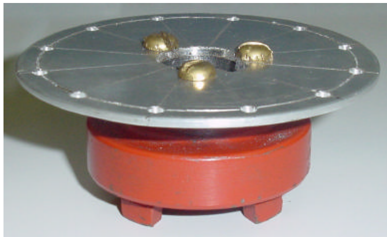
Figure 5-32: Assembled code wheel and drive coupling unit
