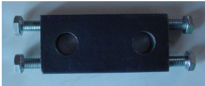
Figure 3-8: Tensioner bolt locator plate
