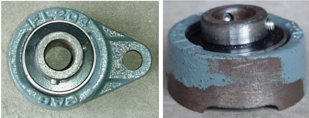
Figure 3-23: Modified self-aligning bearing flanges
