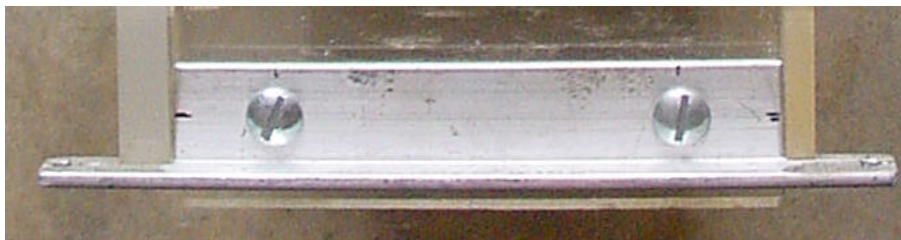
Figure 5-1: Customised aluminium spring mounting brackets
