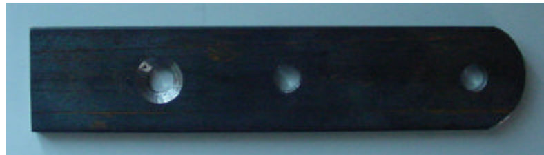
Figure 3-5: Customised side plate of the front sliding axle unit
