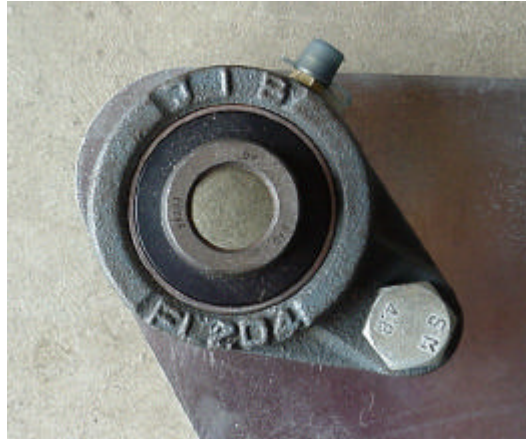
Figure 3-33: Outside face of attached bearing flange
