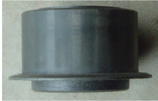
Figure 3-16: Reduced guide pulley for dynamic positions
