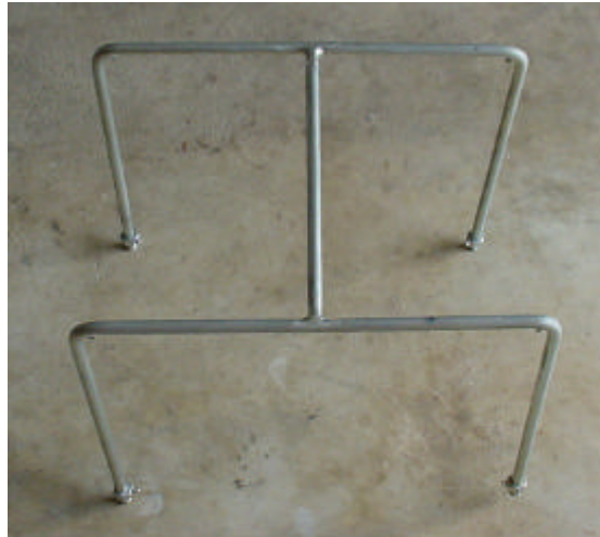
Figure 4-11: Completed computer suspension frame
