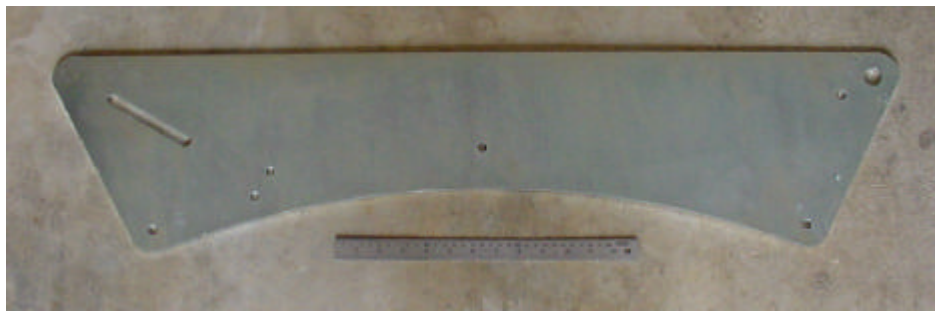
Figure 3-4: Completed internal side plate of track module
