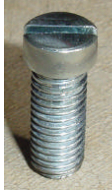
Figure 3-13: Customised bolts for locating the running axles on the front sliding axle, and bogie units
