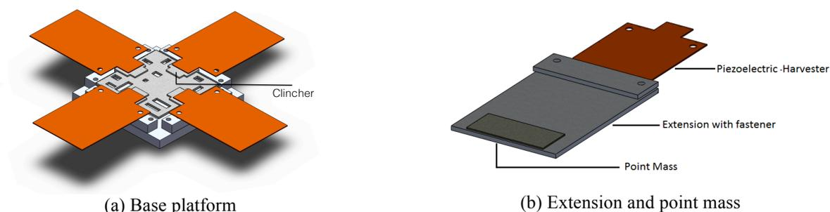
Figure 4. Piezoelectric harvesters mounted on base platform, and extension for lowering resonant frequency
