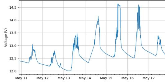
**Fig. 2** Battery degradation and recovery during a storm.
