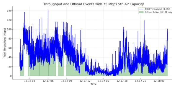
**Fig. 4** Offloading at less than 75 Mbps of throughput.
