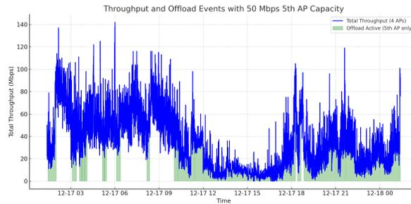
**Fig. 3** Offloading at less than 50 Mbps of throughput.
