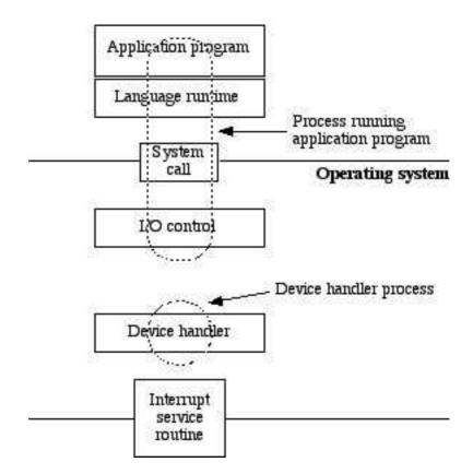
(a) [5 marks] The thread executing in the application program makes a system call to request an I/O operation. Explain the nature of a system call emphasising how it differs from a procedure or method invocation.
