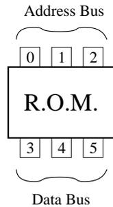
On every clock, the address bus is decoded into an integer *address* between 0 and 7 (following the usual binary representation where e.g. 101 = 5, 011=3, etc). Note, pin 0 holds the *least significant bit*. The *memory* stored at the given address is read, and the data is then written out onto the data bus.
