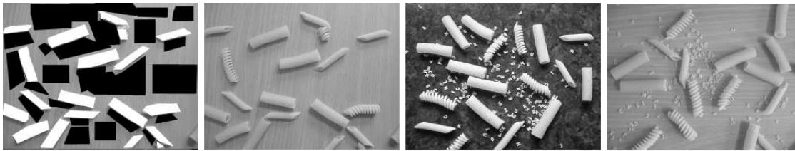
Fig. 6 Pasta training images used to extract training examples. The first image shows the marking to create the examples (white areas are positive examples and black areas are negative examples).
