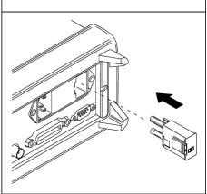
4 Replace fuse holder assembly in rear panel.
