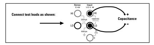
To null-out the test lead capacitance:
