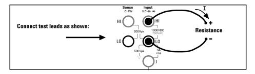
To null-out the test lead resistance:
