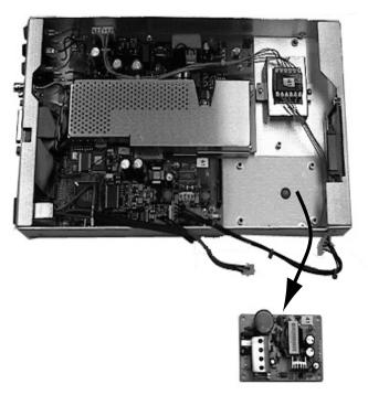
**8 Remove the Display Assembly.** Remove the two Torx screws holding the display bracket to the front panel and lift the display assembly and bracket up and out of the instrument.
