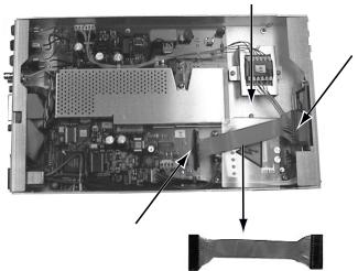
6 Remove the power supply input and output cables.
