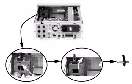
**b** Remove the Torx screw holding the front panel assembly.
