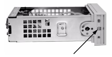
**c** There is now enough play to allow the side of the front panel to be pried from the chassis and removed as an assembly.
