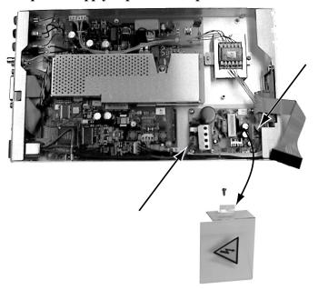
**7 Remove the Power Supply Assembly.** Remove the four Torx screws holding the power supply assembly in place and lift out the power supply.
