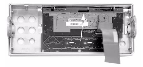
**b** The rubber keypad can now be pulled from the plastic housing.
