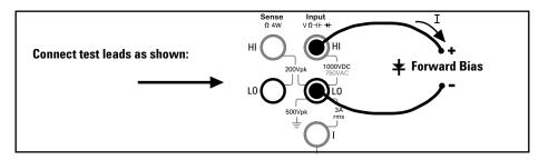
The diode check function is used to indicate correct diode operation; closed-circuit on forward bias and open-circuit on reverse-bias.
