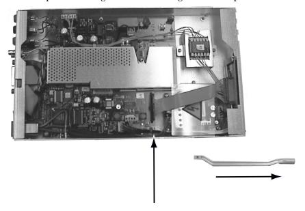
**4 Remove the Display Cable from the main circuit board.** Release the cable connector key from the main circuit board. If desired, remove the display cable by releasing the cable connector key on the *underside* of the display assembly.
